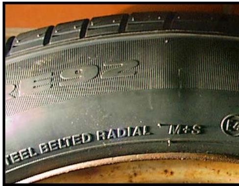
Figure 2: Inflated Tire Sidewall with a “Bulge”
