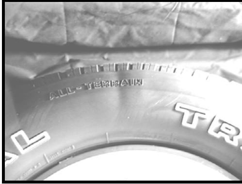
Figure 1: Inflated Tire Sidewall with a “Dent”
